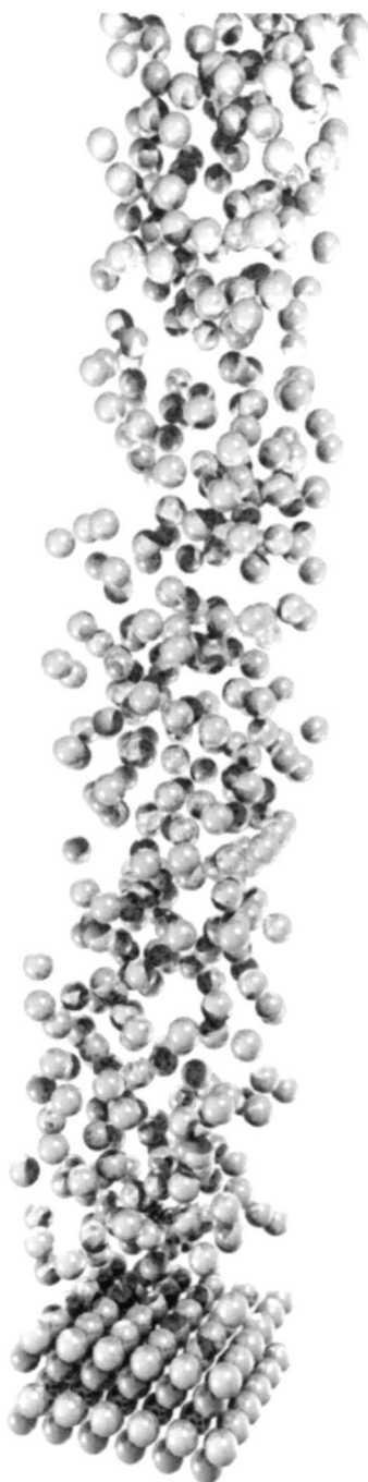
Fig. 3. Start configuration for the simulations of the packing process. The virtual frit consisted of 144 particles which are ordered in four equidistant layers at a distance of two times the particle radius a of each other. The total number of spheres was equal to 600. The unit cell has a length of 15a in the x and y -direction and 122a in the z -direction.
